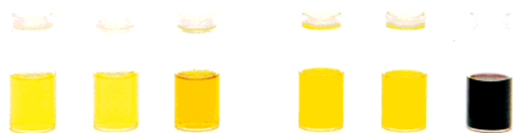
Figure 2. Color changes (if any) induced by the addition of anions. From left to right (dichloromethane solutions): 1 ; 1 + Cl - ; 1 + F - ; 3 ; 3 + Cl - ; 3 + F - . All anions were used in the form of their tetrabutylammonium salts.
